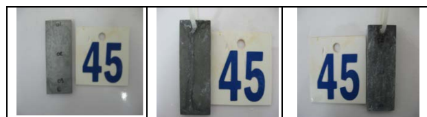
Figure 1. Samples without appearance of corrosion after 2160 hours in salt spray chamber
